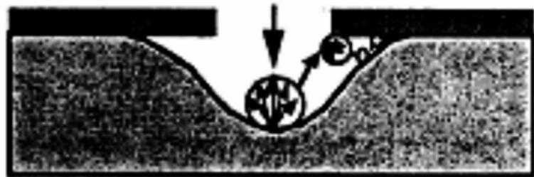
Figure A-4 Atomic Oxygen Undercutting
