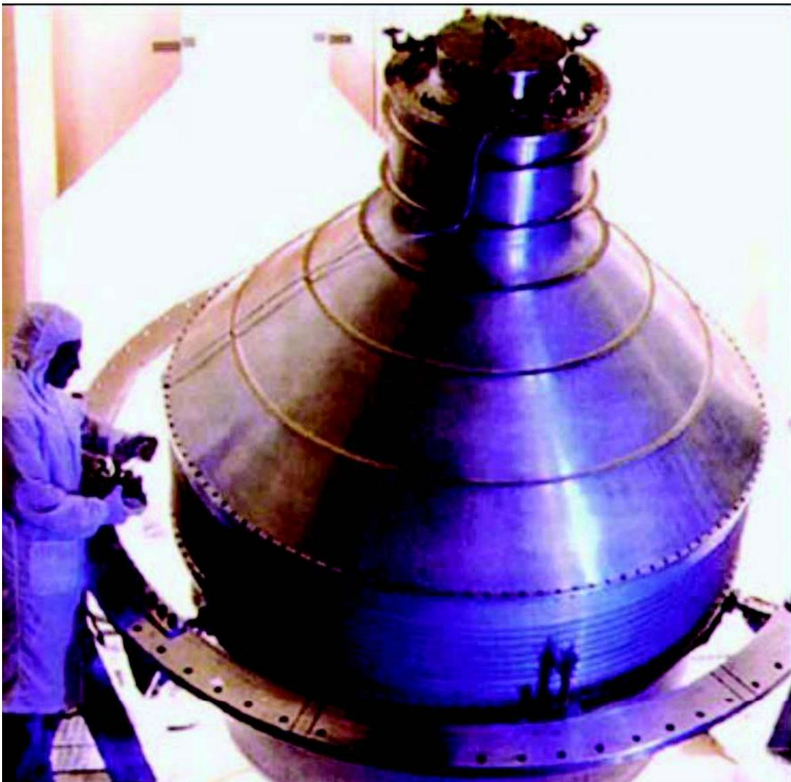
Figure A-2 Gravity Probe B Dewar
